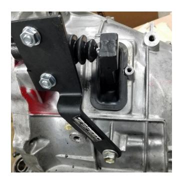
Install Stainless Clutch hose to OEM hard pipe and slave cylinder AND ROUTE AWAY FROM EXHAUST AND STEERING KNUCKLE. Remove the 1 or 2 metal harness brackets (depending on model) from starter harnesses and zip tie harness to slave bracket. You can route the harness between bracket and transmission.
