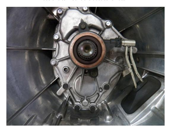
Install CMAK Release Bearing Guide Tube and Retainer plate onto front cover with supplied bolts, YOU MUST USE SUPPLIED BOLTS (Use blue Loctite on threads) in same location as the stock CSC making sure center bearing guide aligns & centers under retainer plate. TQ bolts to factory spec of 80 inch lbs and loctite threads.
