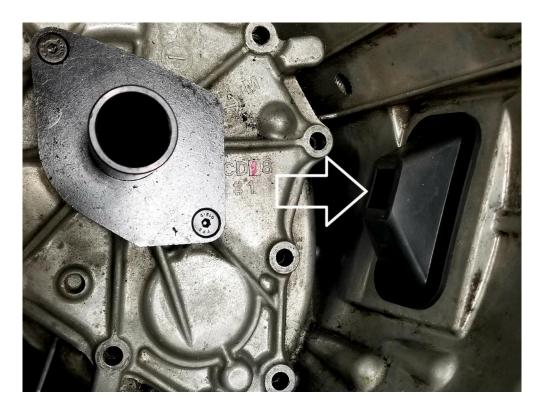
install CMAK Clutch Fork, Bearing and Bracket assembly with the QTY (5) 50mm long bolts, Slip fork and bearing assembly preassembled through dust boot. Adjust boot fitment if needed.
