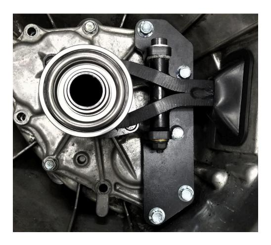
Tighten top and bottom 2 bolts on the bracket finger tight while holding up of fork end slightly. (this centers the bracket) then finger tighten the other 3 bolts, TQ top and bottom bolts to 20 ft-lbs, then tighten remaining 3 bolts to 20 ftlbs. Check fork operation, If throw out bearing does not move easily loosen 5 bolts on bracket and adjust holding slight pressure upwards on slave end of fork, tighten & recheck.
