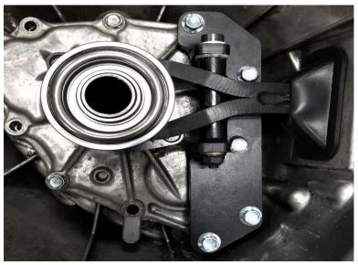
Tighten top and bottom 2 bolts on the bracket finger tight, then finger tighten the other 3 bolts, TQ top and bottom bolts to 20 ft-lbs, then tighten remaining 3 bolts to 20ftlbs. Check fork operation, If throw out bearing does not move easily loosen 5 bolts on bracket and adjust holding slight pressure upwards on slave end of fork, tighten & recheck.
