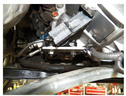
Follow normal bleeding procedures to bleed hydraulic clutch system and ebrake applied test for proper clutch release.
